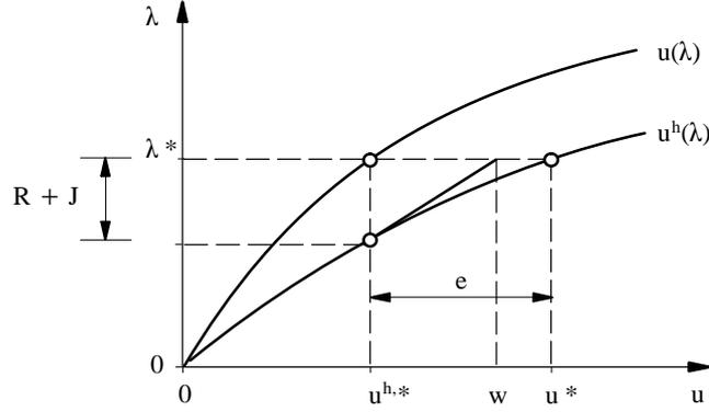
Figure 2: One dimensional example for linearization
