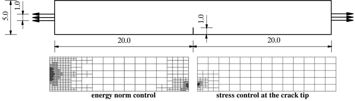
Figure 1: Cracked plate loaded by concentrate forces
