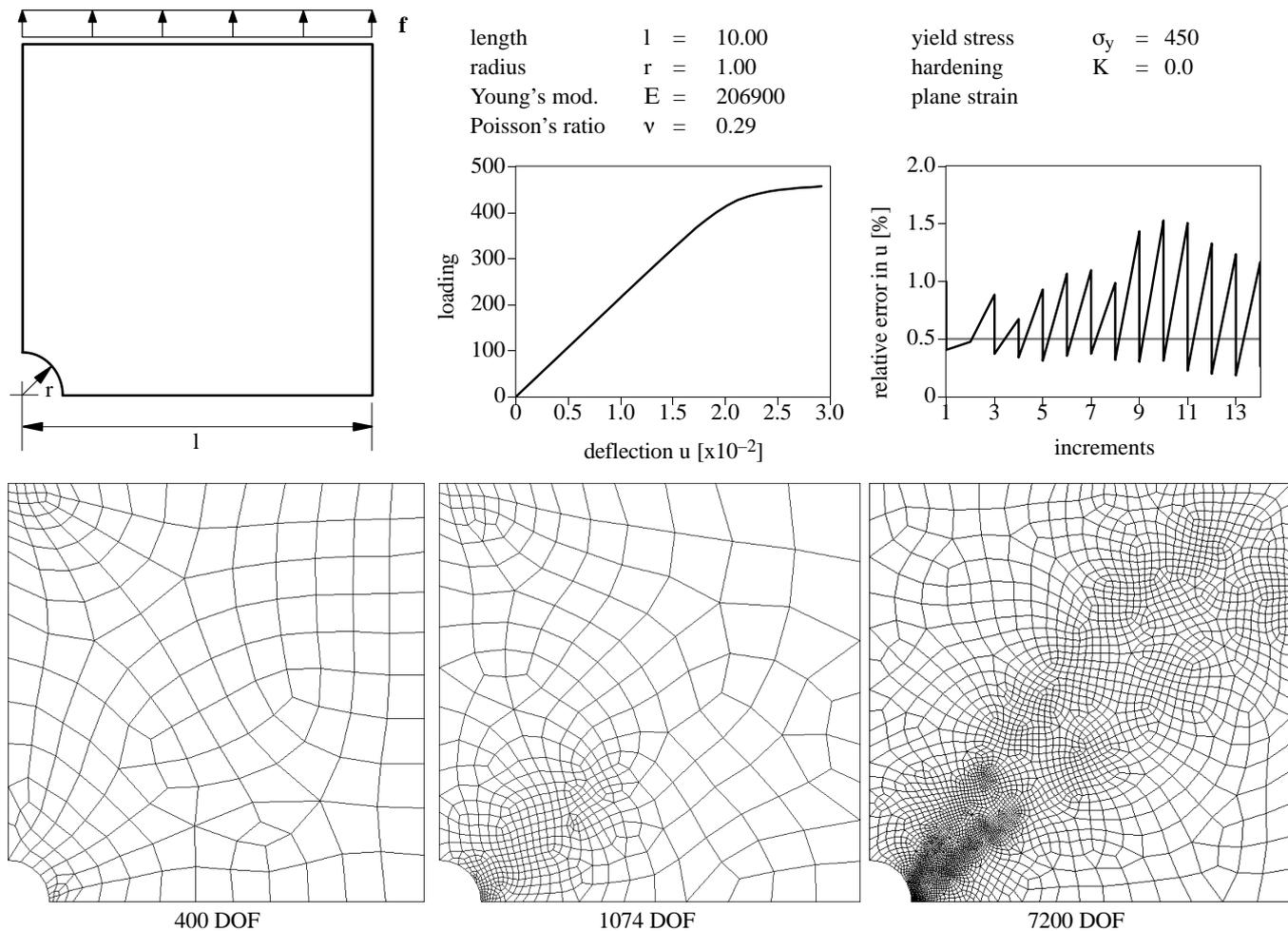
Figure 3: Perforated tension strip: Error control for vertical displacement
